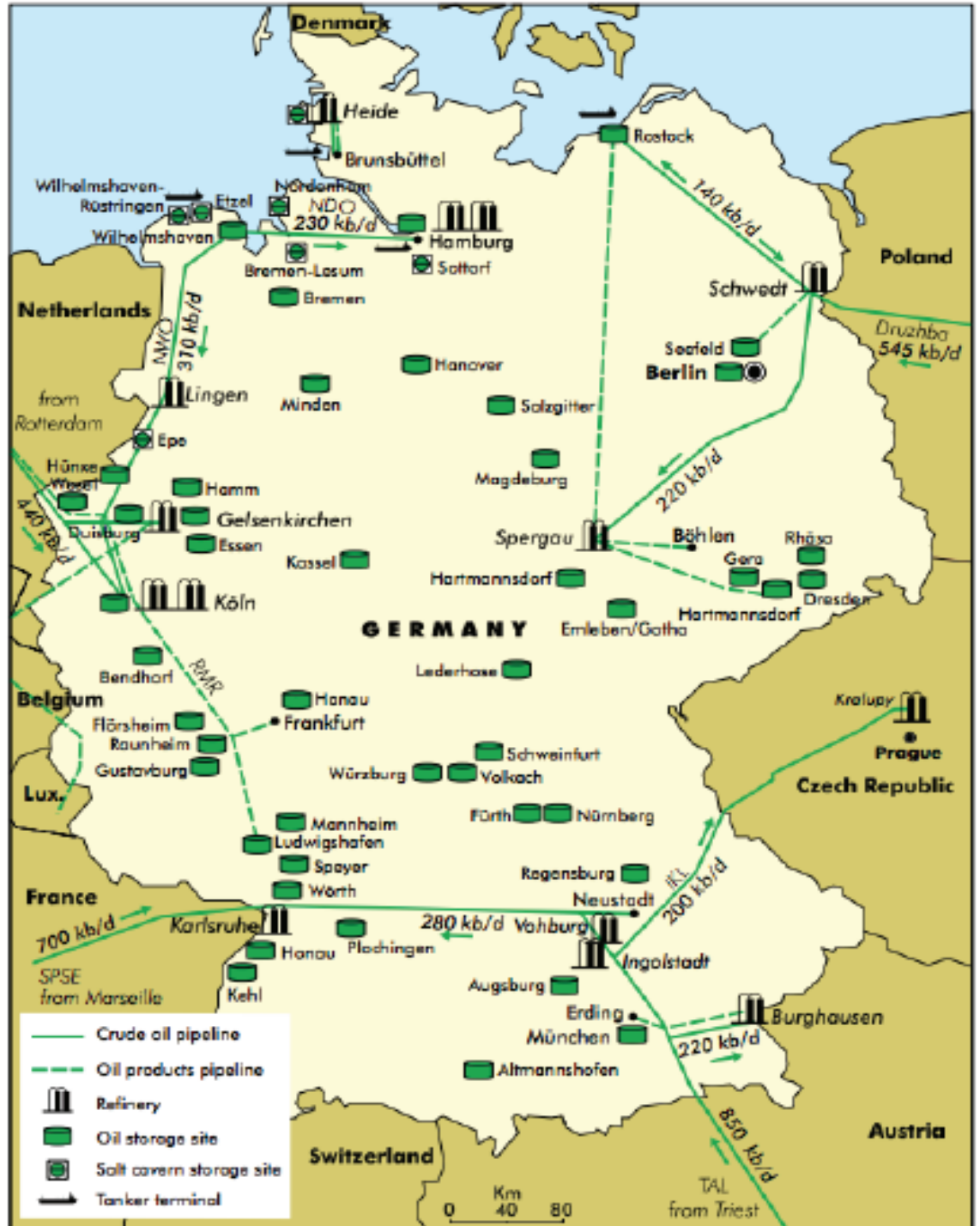
Figure 10: Oil Infrastructure in Germany
